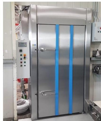
Fig. 8 – Stufa da post-curing
